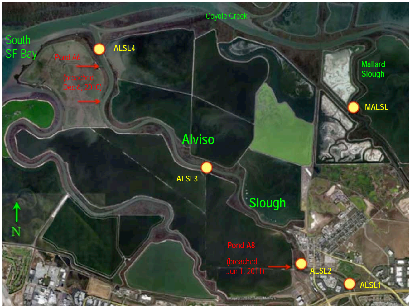
Figure 29. Map of slough fish project area and sampling locations in the South Bay Salt Ponds region. Red arrows show locations of constructed breaches of formerly isolated salt pond A6 and the location of the opening of the Pond A8 Notch.
