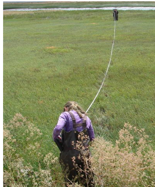
Summer 2010 students measuring 30 X 30 meter polygons to use as sites for validating satellite images.
